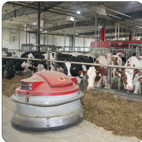
The automated feed pushers ensure food is in close reach for the cows.
